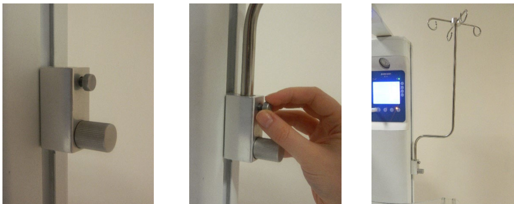
Figure 27. Placing the IV Pole
