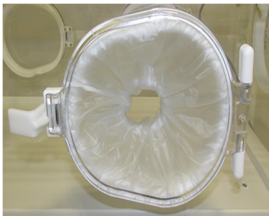
Figure 11. Removal of Iris Ports
