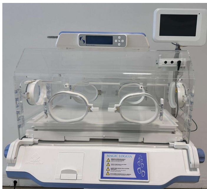
Figure 16: Positioning Blue Angel LED Phototherapy Device on Infant Incubator without Its Stand
