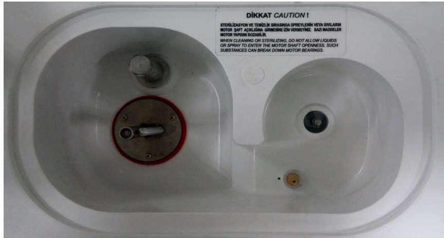
Figure 41: Remaining Surface After Removing the Fan and the Heater
