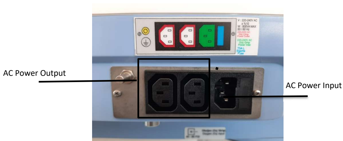
Figure 6: Electric Power Assembly
